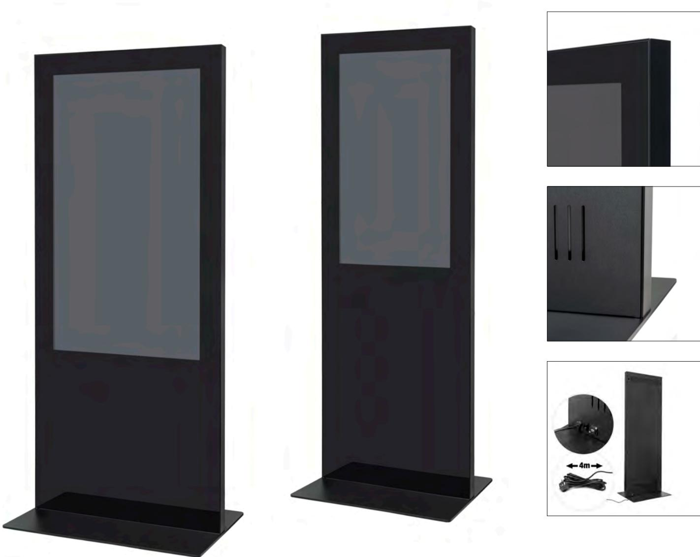
The Digital Info Stand - slim (75mm) made of black aluminum profile, a heavy steel stand featuring (10 mm, powdercoated according to RAL 9016) as well as a front window made of safety glass. The backside is vaulted with a steel sheet, which is secured with two locks and to operate the professional 24/7 LED displays from Samsung can be opened. Available in black.
